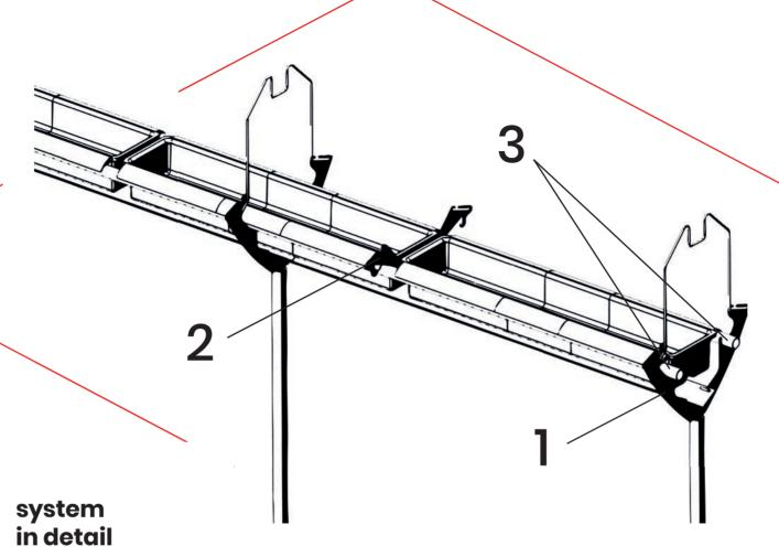
The carrier plates hold the horizontal pipes and already have a recess for a conveyor belt and holes for attaching the irrigation system (micro sprinkler or irrigation hose).
